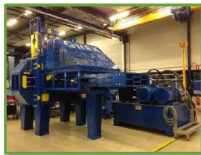
The Organic Extrusion Press (OREX™) separates organic waste into wet and dry waste
